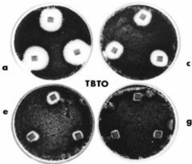
FIG. 2 An *Aspergillus niger* Bioassay of Small-Block Specimens Treated to Selected Retentions With Tributyltin Oxides<sup>9</sup>
